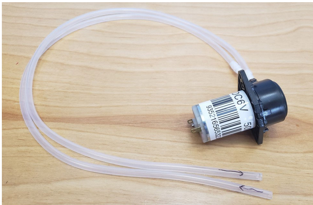
Figure 8. Arrows labeling the direction of water flow in the pump.
